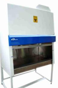
**Biotek** vertical laminar flow class II type B2 biohazard safety cabinets provide personnel and environmental protection. This series of cabinets are referred to as "total exhaust" cabinets because the 100% contaminated air is exhausted to the atmosphere after HEPA filtrations without re-circulating in the cabinet.
